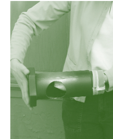
Clean and re-insert the filter cylinder
