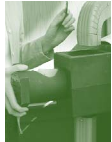
Reinsert the filter cylinder
