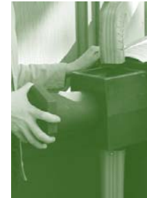
Pull out the filter cylinder
